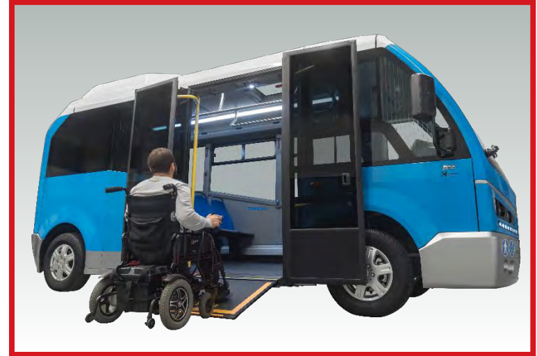
Original low floor with wheelchair accessibility
