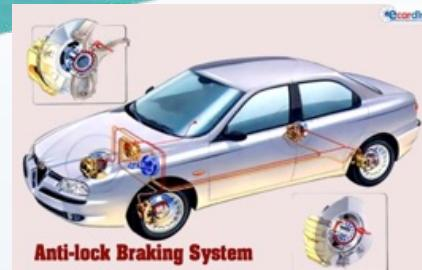
Anti-lock Braking System
